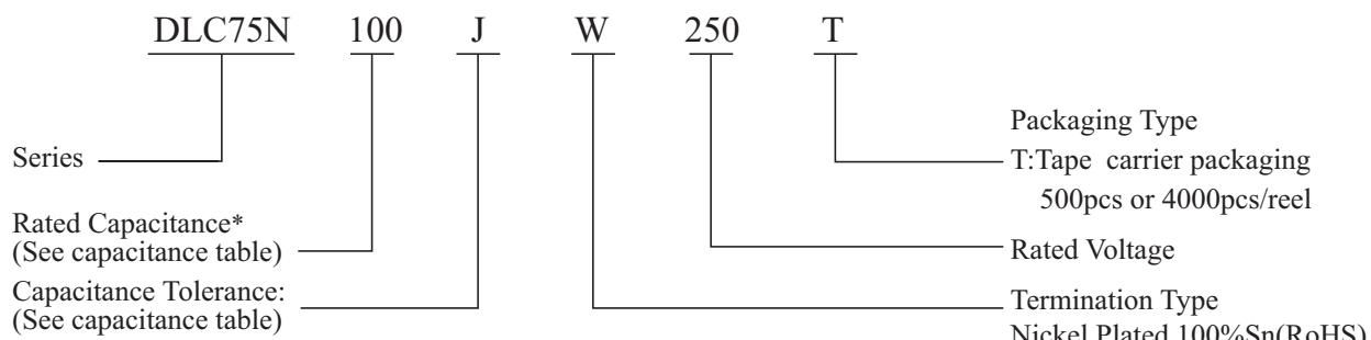
\* When capacitance is less than 1.0, use "R" for decimal
