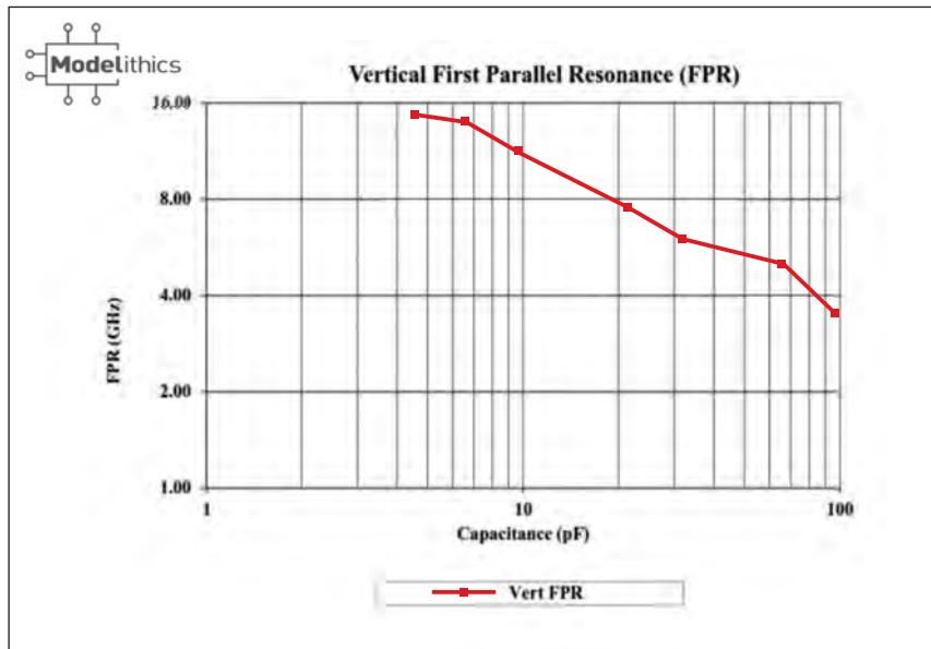
The First Parallel Resonance, FPR, is defined as the lowest frequency at which a suckout or notch appears in |S21|. It is generally independent of substrate thickness or dielectric constant, but does depend on capacitor orientation. A horizontal orientation means the electrode planes are parallel to the substrate.
